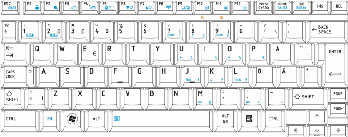
Figure E-16 SW Keyboard layout(Length:276.8mm,Width:112.1mm )
