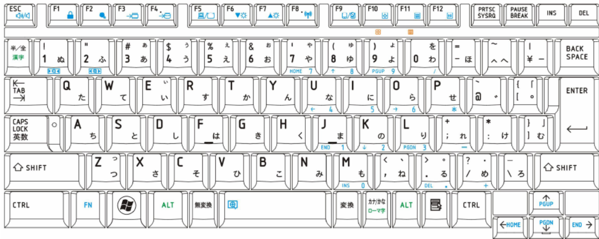
Figure E-19 JP Keyboard layout(Length:276.8mm,Width:112.1mm)
