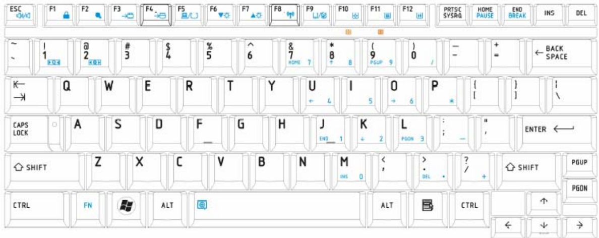
Figure E-1 US Keyboard layout (Length:276.8mm,Width:112.1mm)
