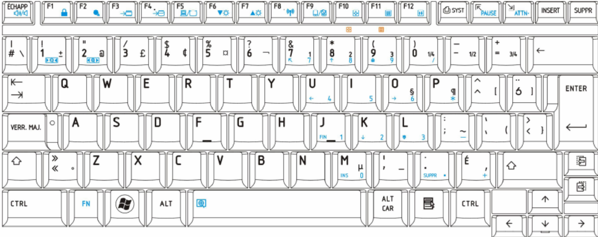
Figure E-15 TC Keyboard layout(Length:276.8mm,Width:112.1mm )
