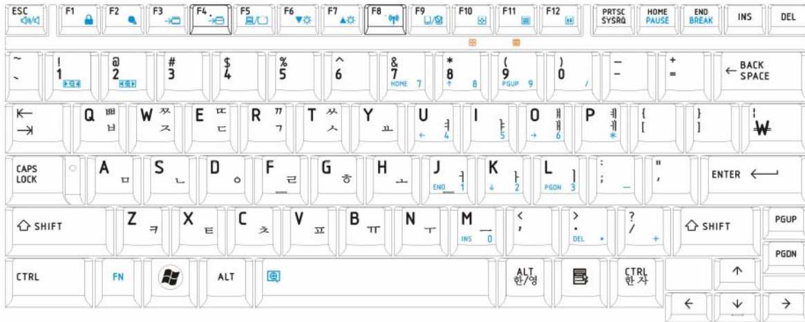
Figure E-12 KR Keyboard layout(Length:276.8mm,Width:112.1mm )
