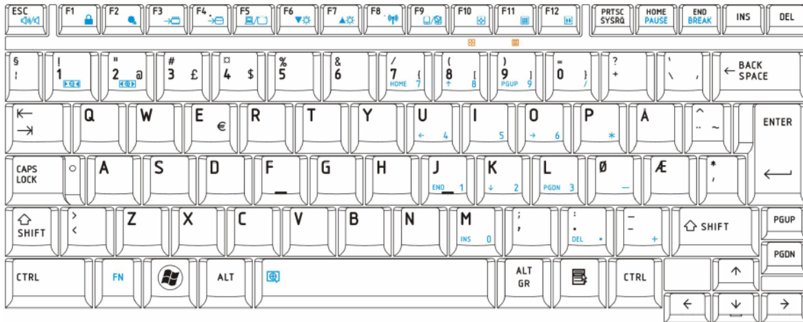
Figure E-13 NO Keyboard layout(Length:276.8mm,Width:112.1mm )
