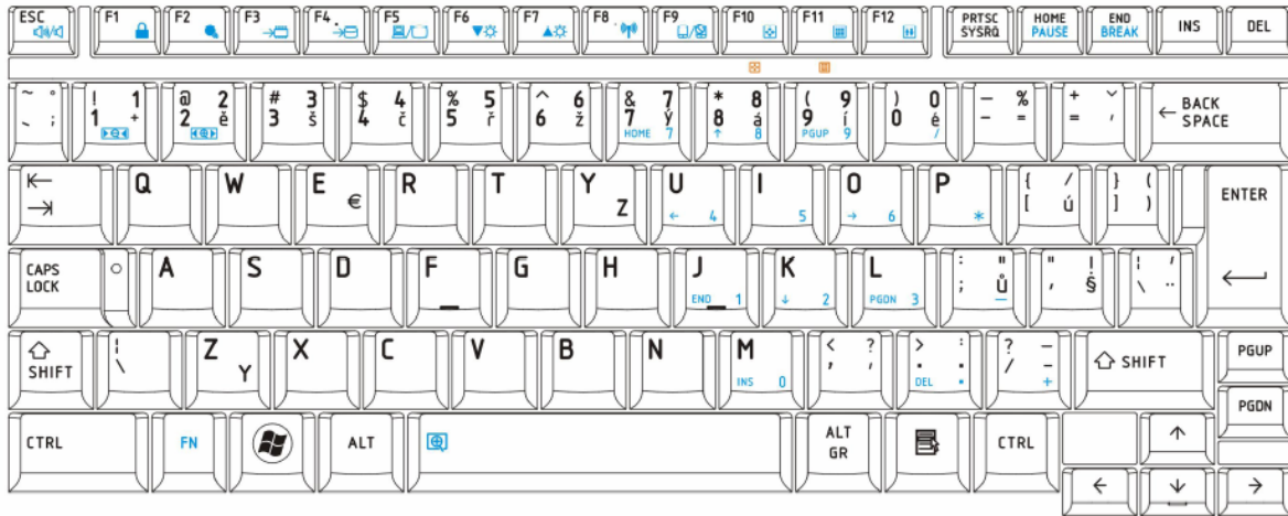
Figure E-5 CZ Keyboard layout (Length: 276.8mm, Width: 112.1mm)
