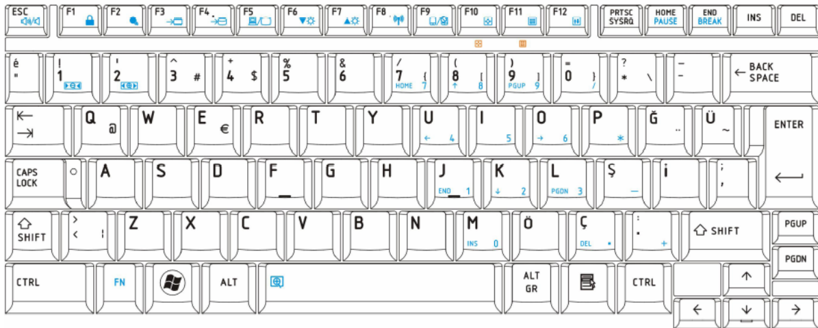
Figure E-18 TR Keyboard layout(Length:276.8mm,Width:112.1mm )
