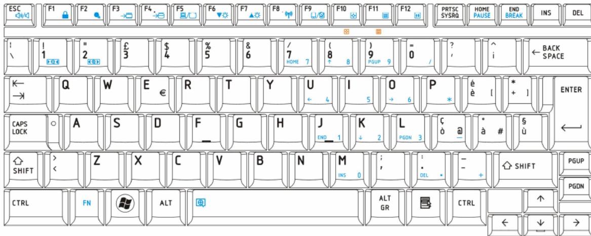
Figure E-11 IT Keyboard layout(Length:276.8mm,Width:112.1mm )
