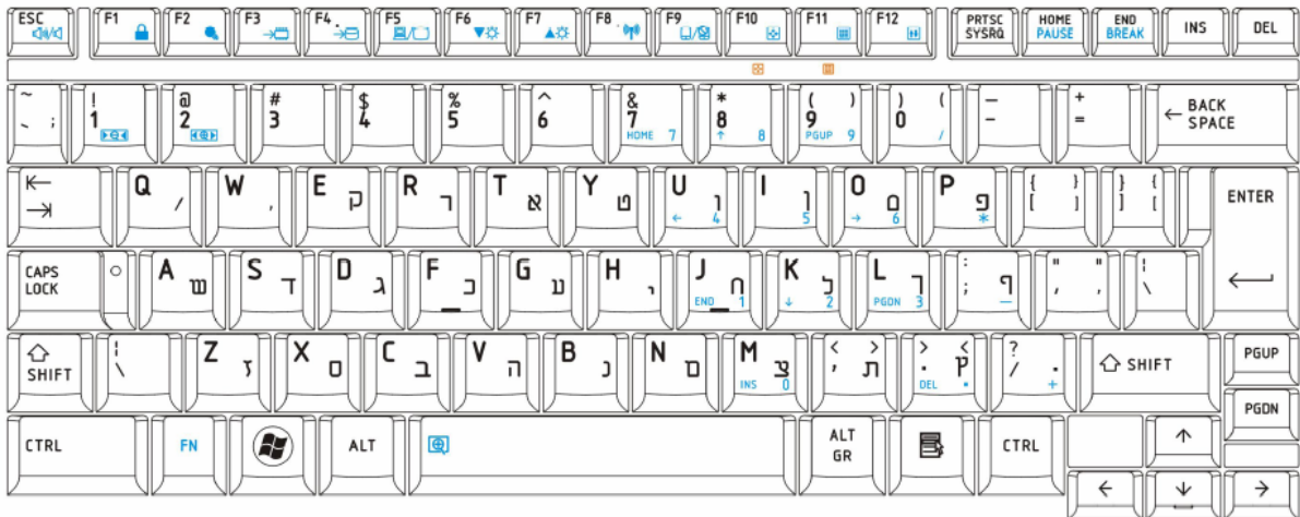
Figure E-21 Keyboard layout(Length:276.8mm,Width:112.1mm )
