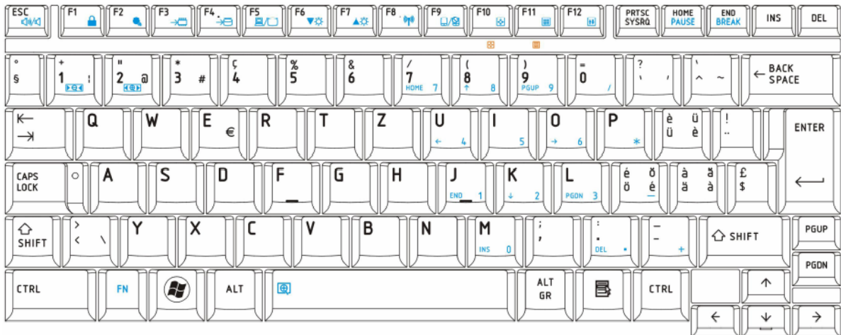
Figure E-20 SL Keyboard layout(Length:276.8mm,Width:112.1mm)
