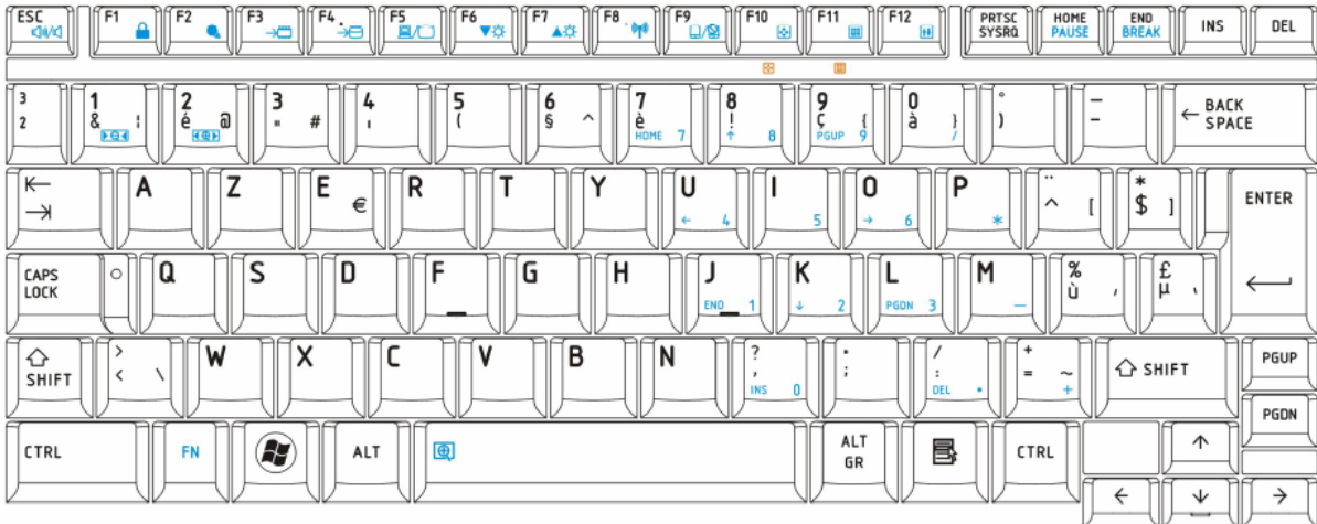
Figure E-4 BB Keyboard layout(Length:276.8mm,Width:112.1mm)
